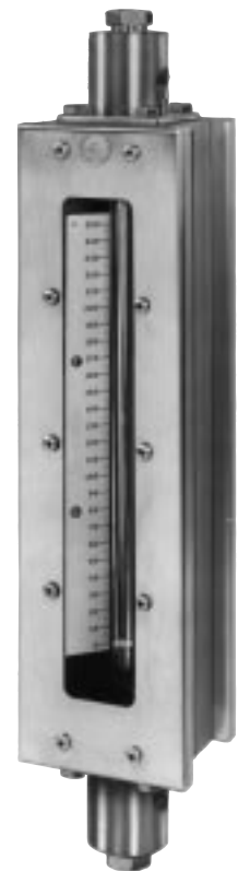
Fig. 4. Type 20-5100 Rotameter has stainless steel case and covers. Connections are threaded. End fittings available in stainless steel, PVC, Kynar or other corrosion resistant materials.
