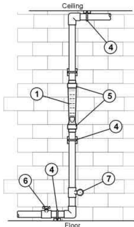
6. Valves - Avoid a system that will impose a sudden burst of flow to the meter. Such a burst will cause the float to impact the float stop with destructive force. Magnet, solenoid, or other quick opening valves cannot be used unless meter is protected against sudden bursts of flow.
