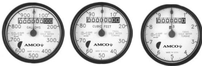
**Magnetic Drive.** The magnetic drive design eliminates miscoupling associated with right angle drives. Torque is absorbed in the undergear assembly below the driving magnet. Consequently, the driving magnet at all flows is turning slowly, assuring magnetic coupling with the register assembly. The undergearing is protected by an appropriately filtered encasement.
