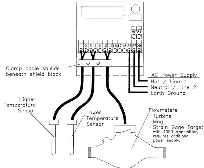
**Wiring Terminal Functions**
