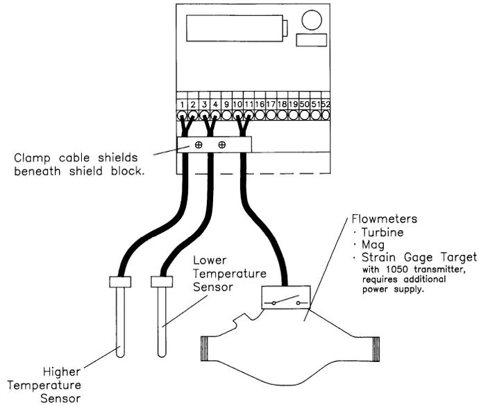
**Wiring Terminal Functions**
