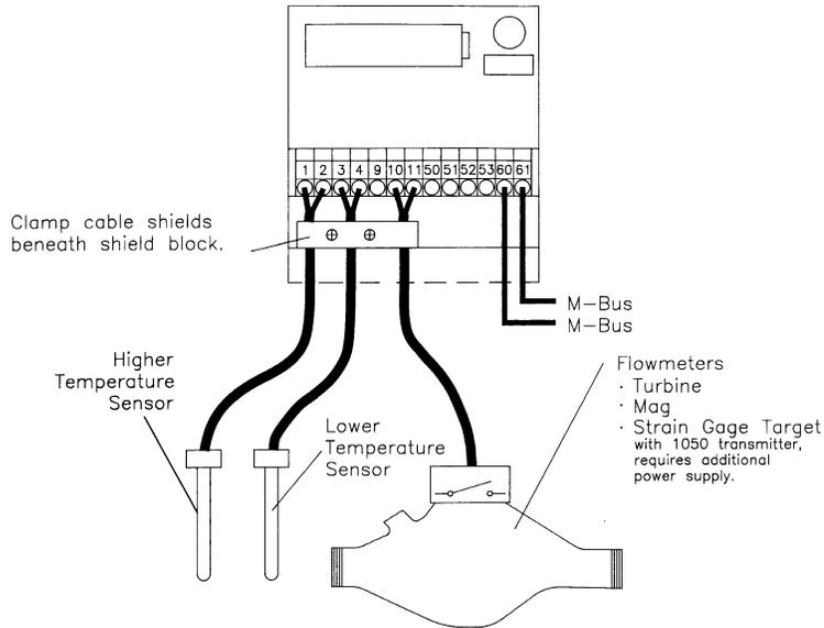
**Wiring Terminal Functions**
