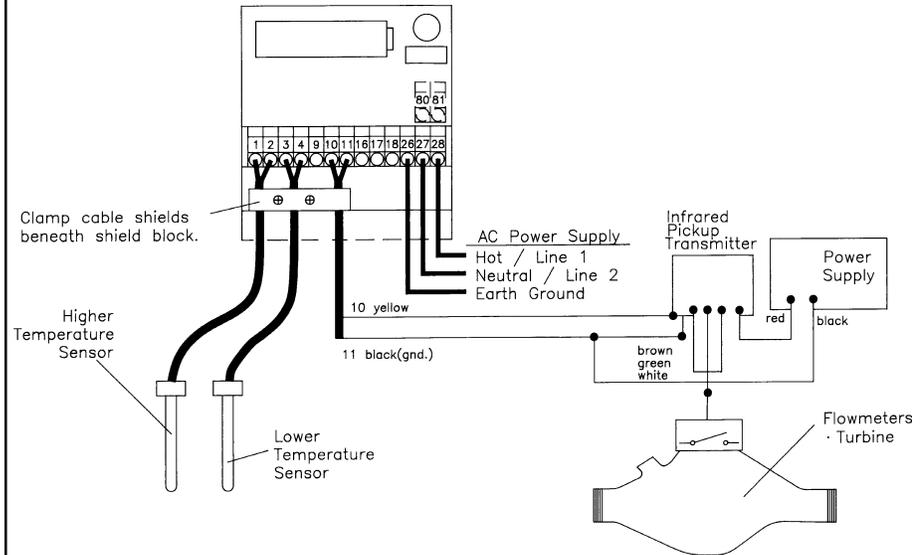
**Wiring Terminal Functions**
