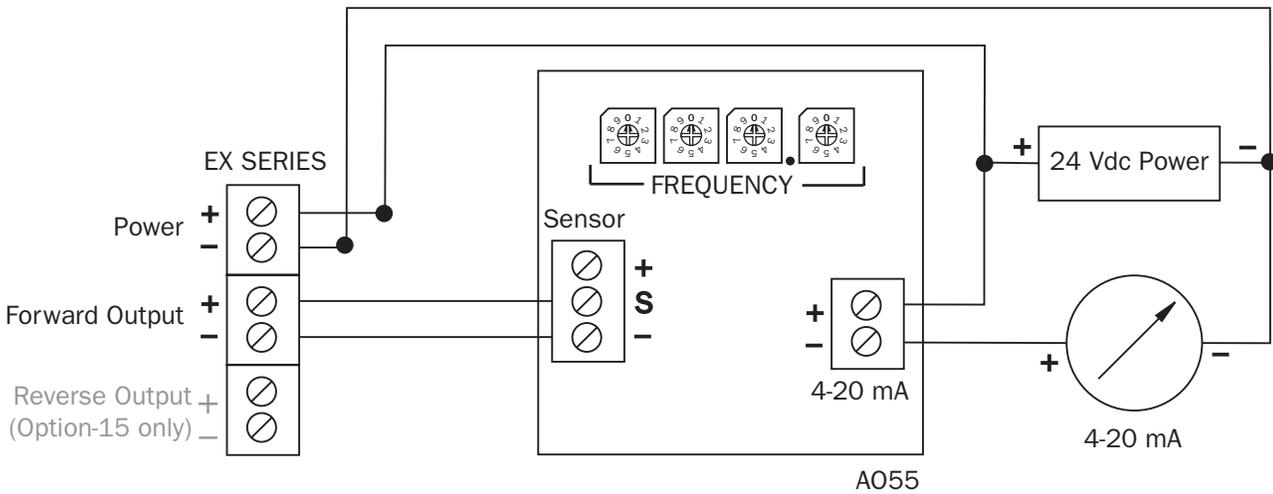
\*See Dual FT420 Diagram for an example of bidirectional connections.
