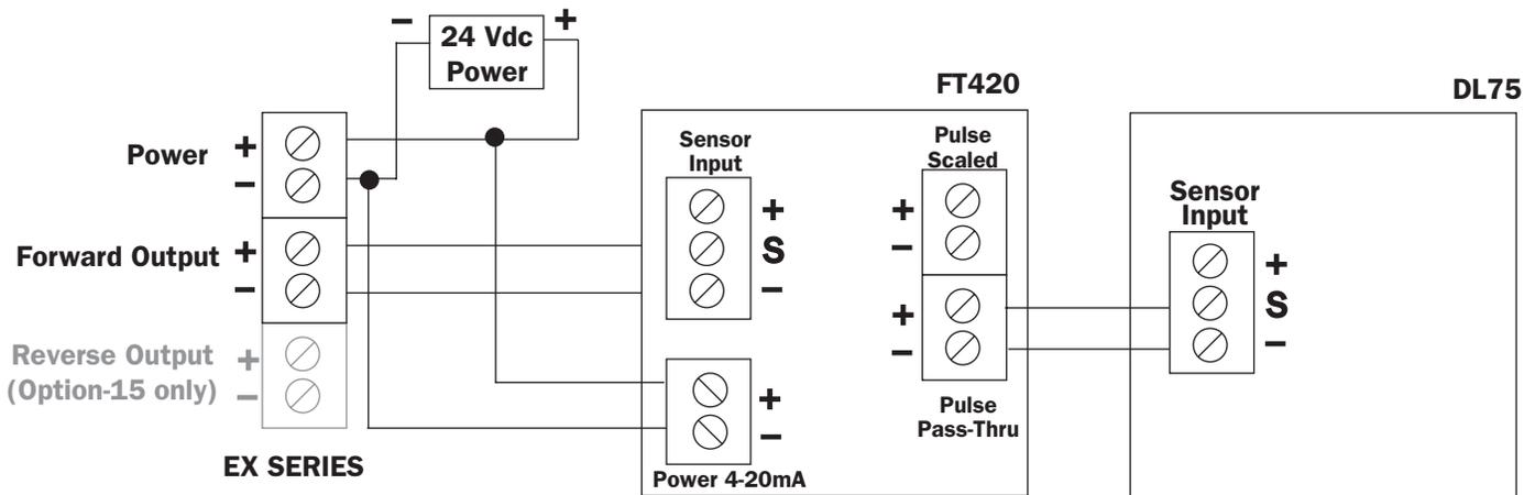
\*See Dual FT420 Diagram for an example of bidirectional connections.
