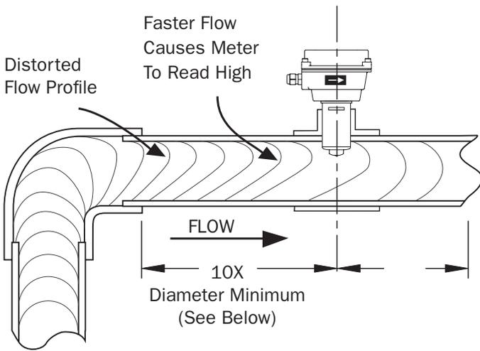
**Fitting Installation.** EX80 Series meters require special fittings. The meter fitting must first be installed in the pipeline. Straight pipe of at least ten times the diameter upstream of the meter and five diameters downstream is strongly recommended in order to achieve proper accuracy. These are minimum values. As the diagrams on the next page will show, you may need more straight run under specific adverse circumstances.
