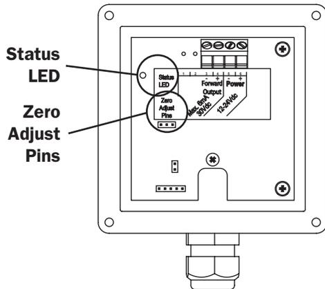
To perform the adjustment, after determining that there is a full pipe with no flow, short between the two pins marked “Zero Adjust”. A red LED light will come on for approximately 50 seconds and then go out. The zero adjustment is completed.
