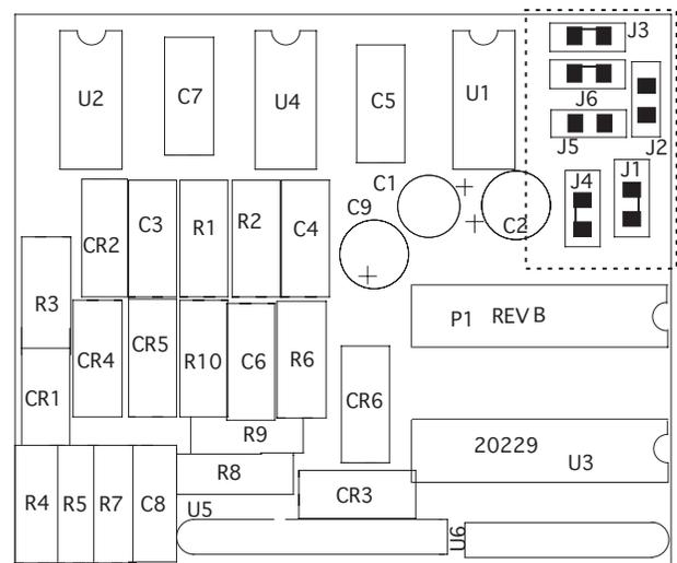
If the unit has the millivolt input bd.# 20229, A & B inputs can be separately solder jumper programmed to accept either a low millivolt or 4-30 V input. Each unit shipped is programmed according to part number. If solder jumpers are made, the part number should be modified to reflect the changes made
