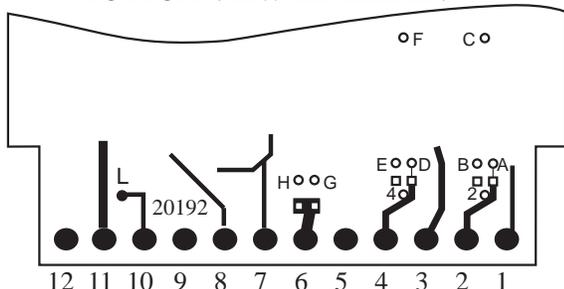
\* The unit must be removed from the case to access jumpers C & F, all other jumpers can be accessed by removing the plastic extender.
