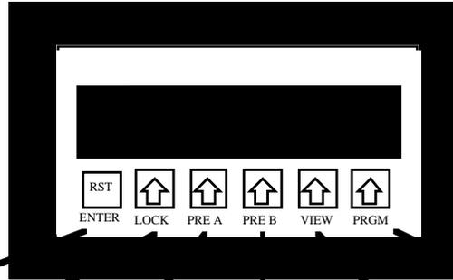
Press to "reset" in operating mode. Press to "enter" in programming mode.
