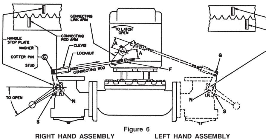
**To Adjust the Valve Connecting Rod**
