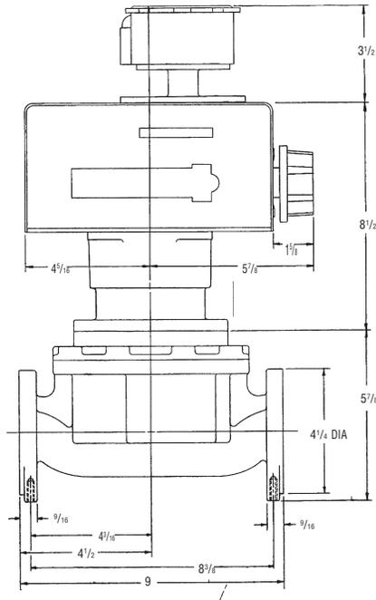
ALLOW 2 INCH CLEARANCE FOR REMOVING REGISTER
